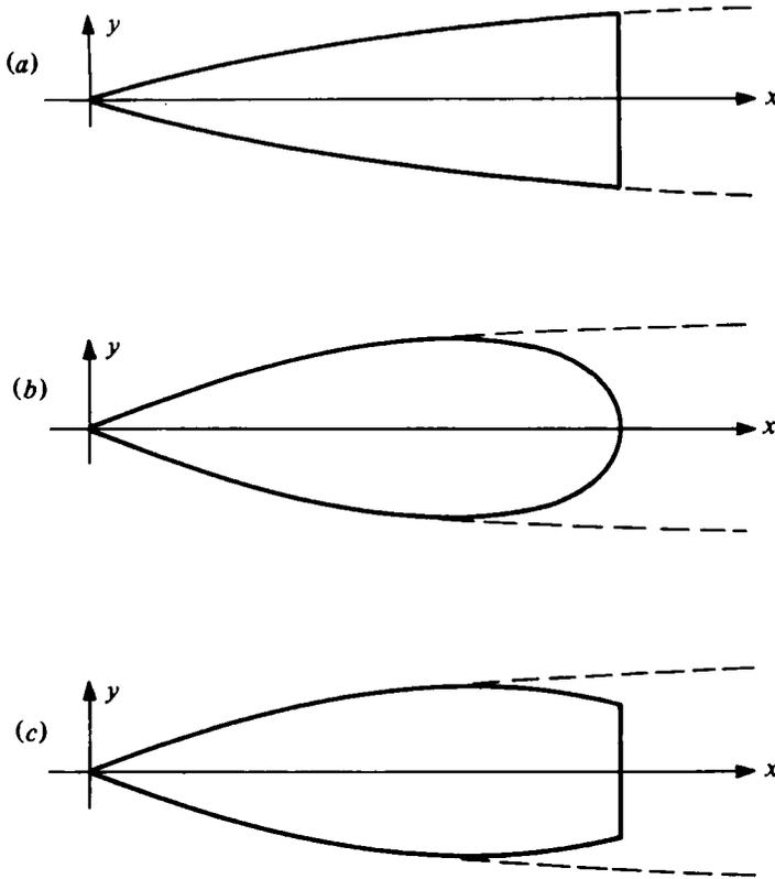
FIGURE 2. Planforms of lifting surfaces with (a) abrupt trailing edge, (b) swept trailing edge, and (c) combination of abrupt and swept trailing edges. Dashed lines denote typical positions of the outboard edges of the trailing vortex sheet.
