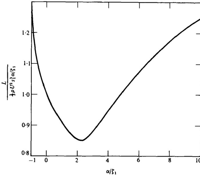
FIGURE 3. Normalized lift-slope coefficient for a planar delta wing with unit chord length, base span  $s_1$ , base elevation  $\zeta_1$ , and angle of attack  $\alpha$ .
