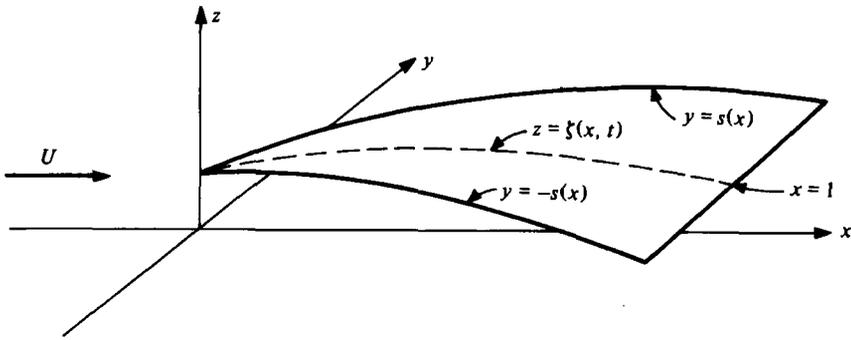
FIGURE 1. Definition of the co-ordinate system and lifting surface in close proximity to the ground-plane  $z = 0$ .
