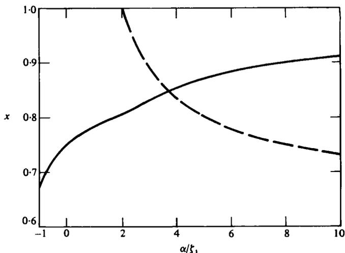
FIGURE 4. Centre of pressure (—) and transition point  $x_*$  between leading and trailing edges (---) for a planar delta wing.
