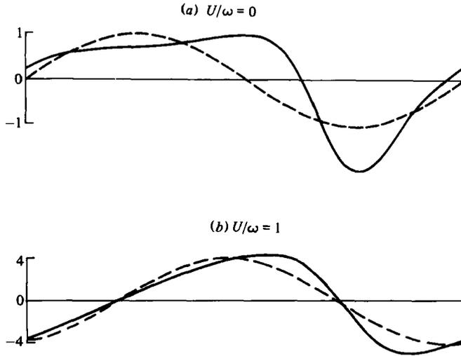
FIGURE 5. Unsteady lift coefficient (26) vs.  $\omega t$  in the interval  $(0, 2\pi)$ . The solid curves are for a sinusoidal heave amplitude equal to half the mean elevation and the broken curves are the corresponding linearized results.
